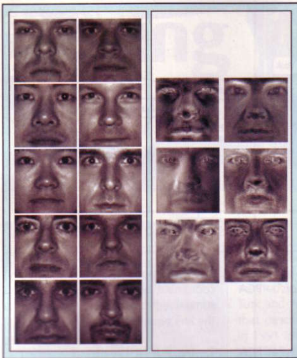
FIGURE 3. Left: Face images for 10 people. Right: The first six principal components viewed as eigenfaces.
